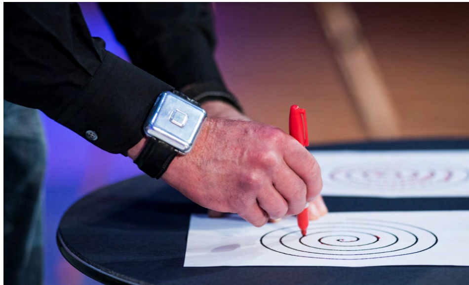
The wearable device developed by Encora Therapeutics uses vibrations to send signals to the brain that can help relieve tremors of the hand. Credit: 2.009 Team
