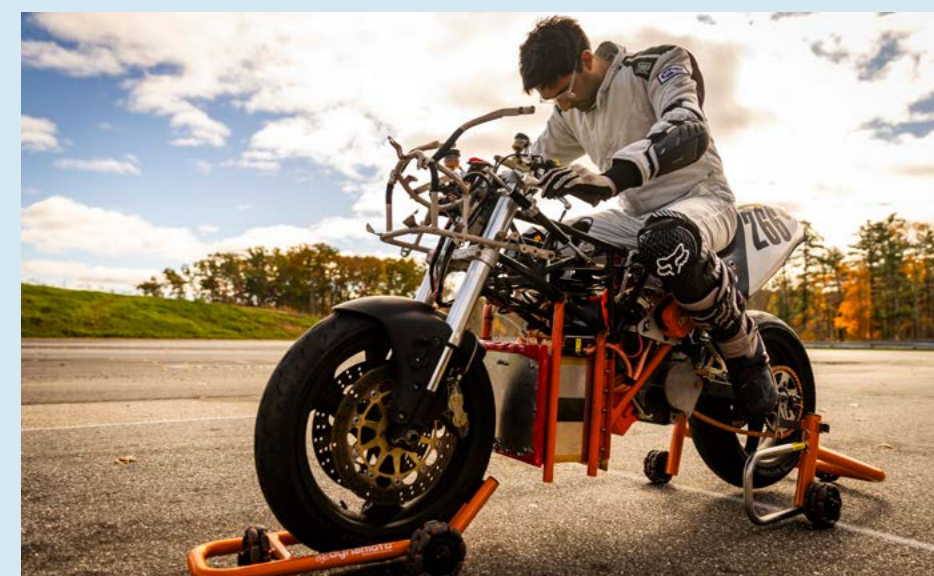
Aditya Mehrotra is designing one of the first-ever hydrogen-fuel-cell-powered motorcycles realized in real hardware and tested on the road and racetrack. Mehrotra and his team want to build a truly green vehicle that has the same performance, range, and practicality as a gasoline vehicle with none of the harmful emissions. Credit: Adam Glanzman
