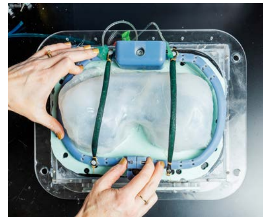
A soft, robotic, implantable ventilator developed by Ellen Roche and her colleagues. Credit: M. Scott Brauer
