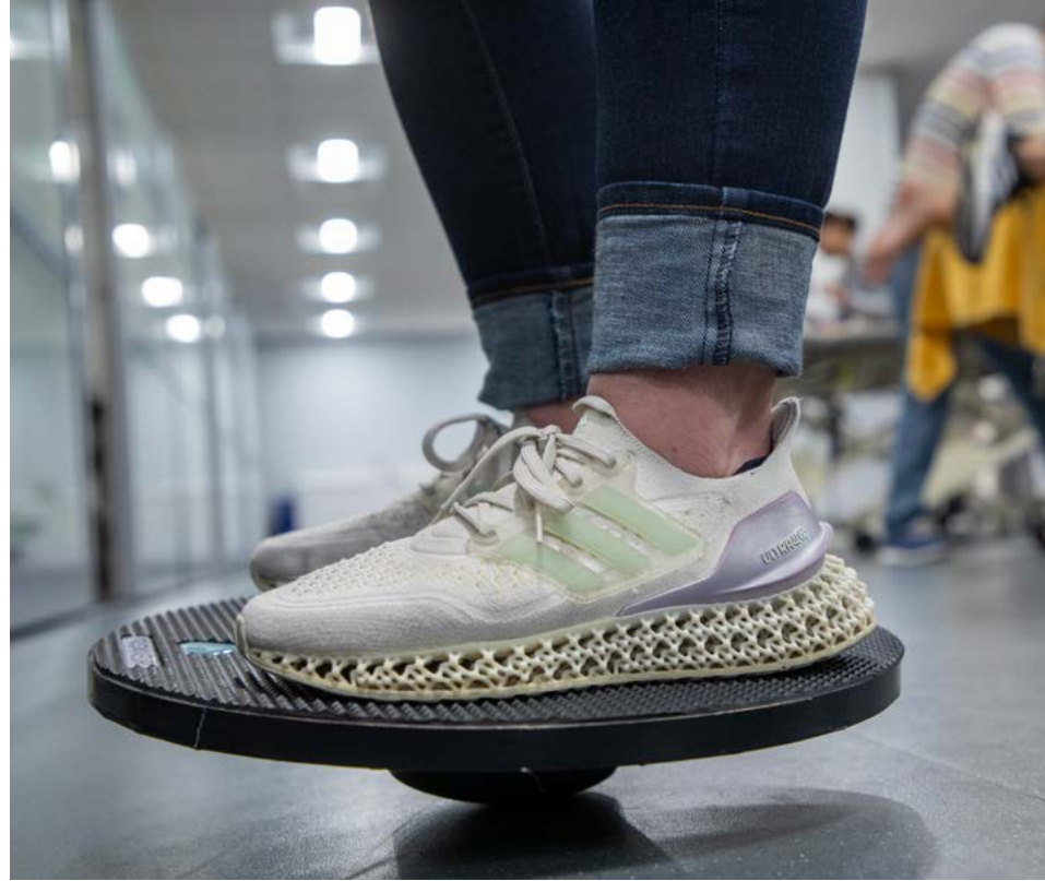
An instrumented balance board is used to gamify the recovery process for lower limb injuries and target the injuries' effects on the body's movement control systems. Credit: John Freidah
